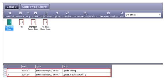
If you update the controllers configuration such as privileges or door-delay etc., you must upload to the controllers.
