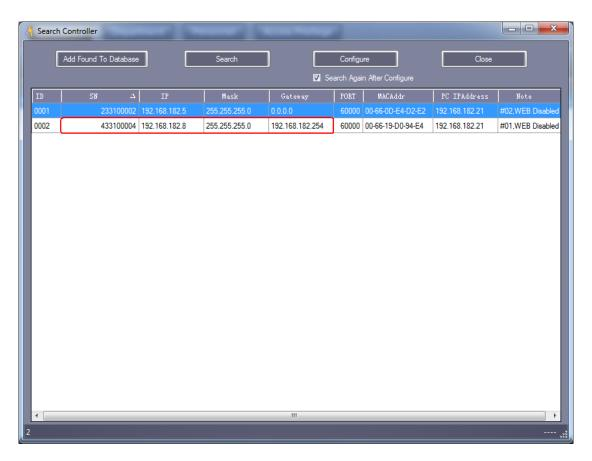
After IP address setting, you can move to chapter <u>2.2.1 Add/Set up Controller</u> to set the controller parameters, the IP address should be assigned to the corresponding Controller.
