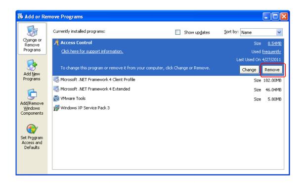
Find software "Access Control" in "Currently installed programs", Click "Remove".
