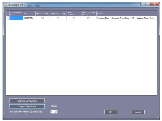
"Threat Code": Must be used with the PIN keyboard Card Reader.
