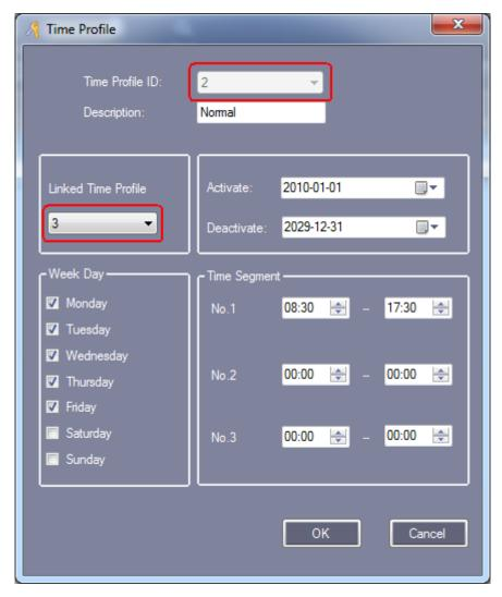
After setting "Time Profile", you need to assign permissions to the corresponding user in the Access Privilege, and then the users can pass in and out at the specified "Time Profile".
