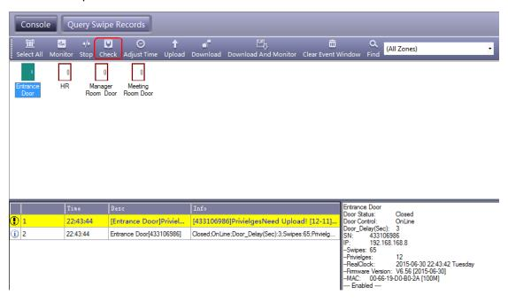
It will show the controller's basic information .such as the amount of swipings and privileges, Door status, control status, open delay (sec) .lf the controller is well communicated with computer, the door label's color is green, otherwise the color is red.
