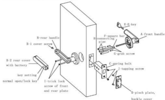
Diagram of Door Lock Installation
