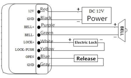
Remark: Jumper Cap on NC terminal for Power Off unlocking and NO terminal for Power ON unlocking (in this case please set Unlocking Duration to be [00]).
