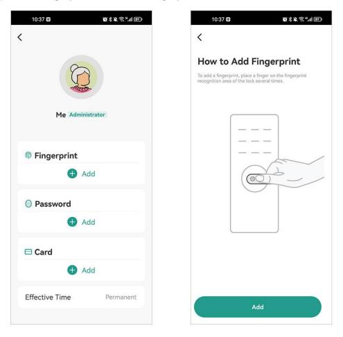
Place fingerprint on the access control machine 3 times. Add fingerprint successfully, click "OK"
